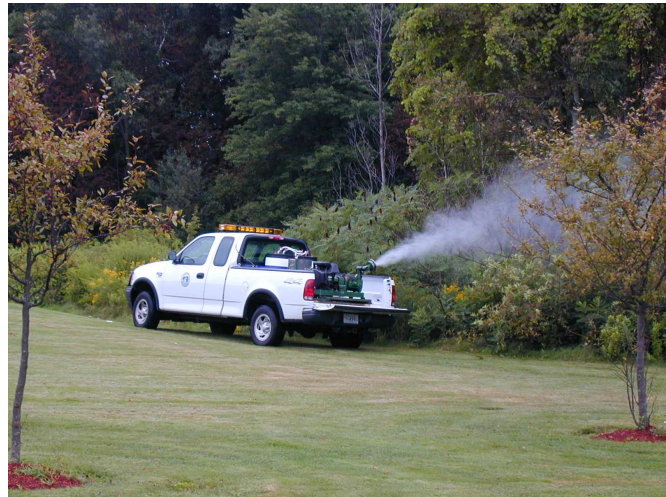
Figure 24. Truck applying barrier treatment.
