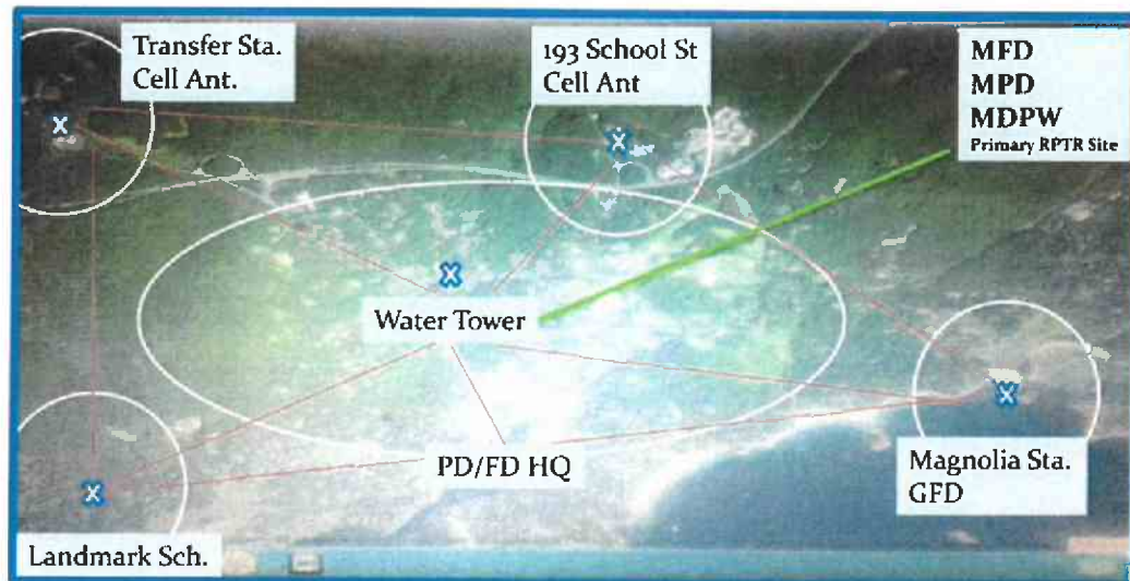
FIGURE 30: MANCHESTER COMMUNICATIONS SYSTEM WITH CO-LOCATED TRANSMISSION AND RECEIVER SITES ON THE WATER TOWER Diagram courtesy of Manchester Fire Department
