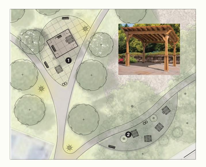
**PHASE F:**  $\sim$ 1,500 sf paved plaza with 10'x20' monoslope cedar pavilion in New England rural architectural style, accessible wood picnic tables and benches, trash and recycling receptacles, accessible connections to new asphalt paved park path system, shade trees, and flowering tree plantings
