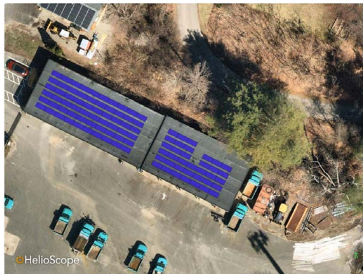
Preliminary Design of 46 kW Solar Array on DPW Roof
